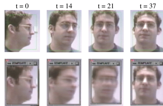
Figure 7: The IIR filter. As the image changes from a face in profile to a frontal view, the template is updated using an IIR. If the image is stable for some time, the template also remains stable.
